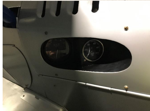
RPM and Oil gauges are located in the engine nacelles.
